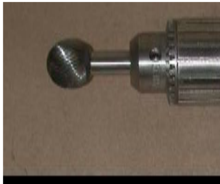
Figure 6: Photograph of typical spherical carbide ball burr
